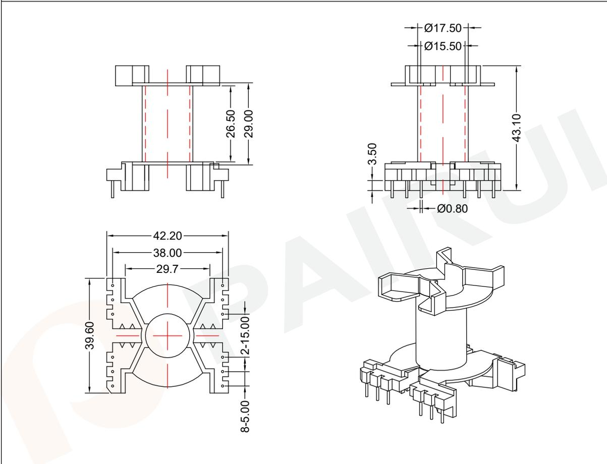
Winding data and area product for 12-pins PQ40/40 coil former
